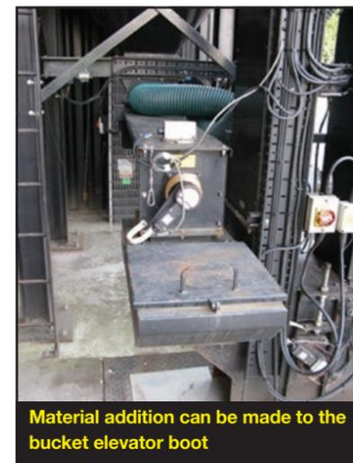
**Material addition can be made to the bucket elevator boot**
