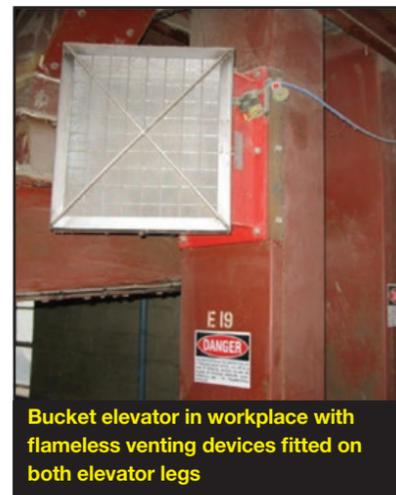
**Bucket elevator in workplace with flameless venting devices fitted on both elevator legs**
