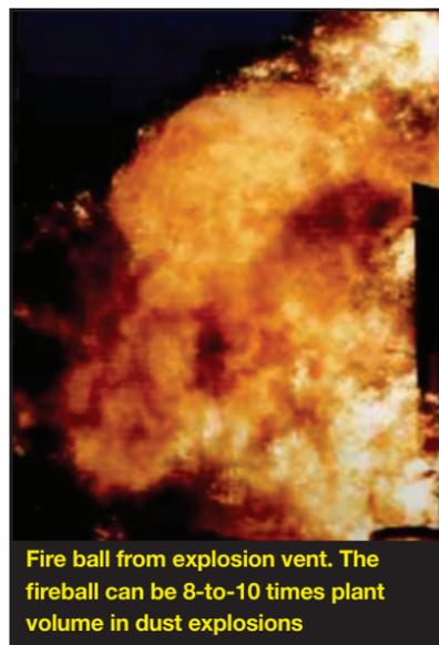
**Fire ball from explosion vent. The fireball can be 8-to-10 times plant volume in dust explosions**
